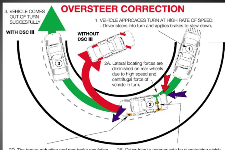
2D. The torque reduction and rear brake regulation should stabilize the vehicle at this point. If not the left front wheel has a high degree of lateral locating force and is momentarily regulated.
