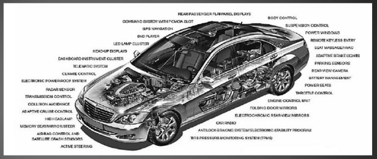
Mechatronic sophistication in automotive vehicles is increasing. For example, Mercedes S-Class employs at least 70 networked ECUs (electronic control units).Ten years ago, most automotive vehicles had three ECUs. Safety & Convenience Including: Stability sensing Pedal positioning X-by-wire
