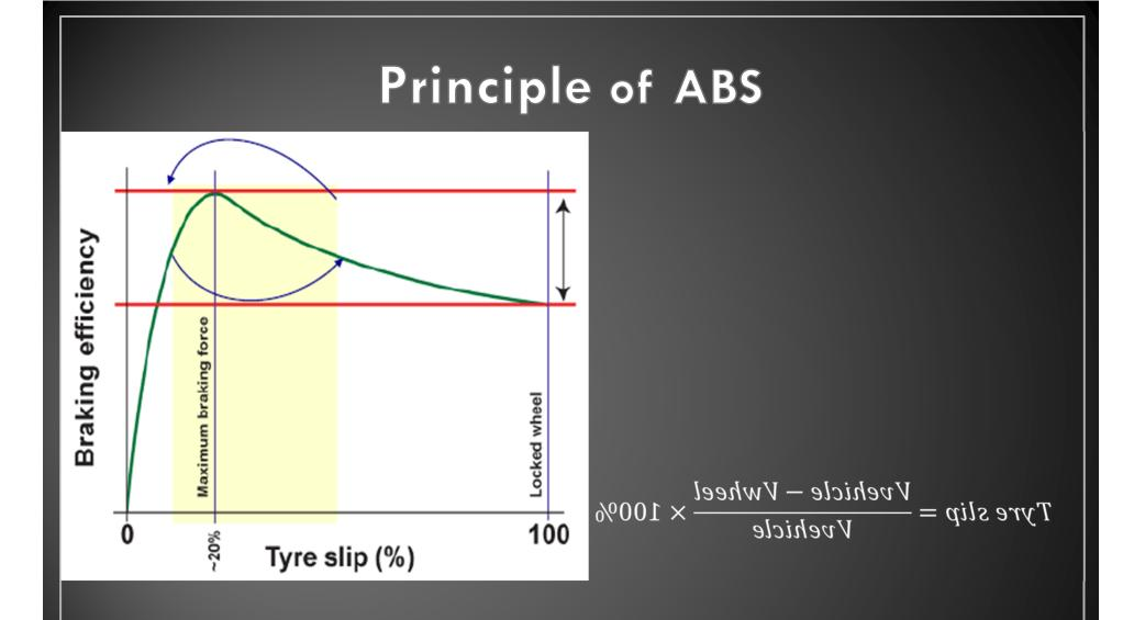
During emergency braking, ABS automatically cycles tire slip around point of maximum braking efficiency
