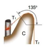
Since area does not affect the developed friction for a belt, the formula for flat belts is applicable to round line. Only angle of wrap and coefficient of friction govern developed tension
