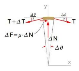
Incremental forces ΔN and ΔF develop as a result of the applied incremental tensions. By performing an equilibrium analysis:
