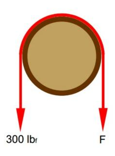
Line wrap is 180° or π radians. When lifting, force F is the tightside of the line (T<sub>2</sub>). To solve for T<sub>2</sub>:
