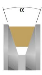
The friction developed by a V-belt can be developed in a similar fashion. The relationship between tightside and slackside tension for a V-belt is:
