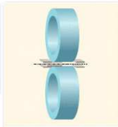
Through feed grinding
