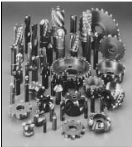
FIGURE 12.8: A variety of indexable milling cutters. (Courtesy Ingersoll Cutting Tool Co.)
