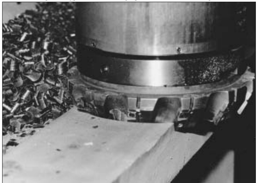
FIGURE 12.1: A typical milling operation; the on-edge insert design is being used. (Courtesy Ingersoll Cutting Tool Co.)
