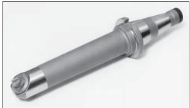
FIGURE 10.1: Adjustable boring bar for precision holes. (Courtesy: National Acme Co. Div. DeVlieg-Bullard, Inc.)
