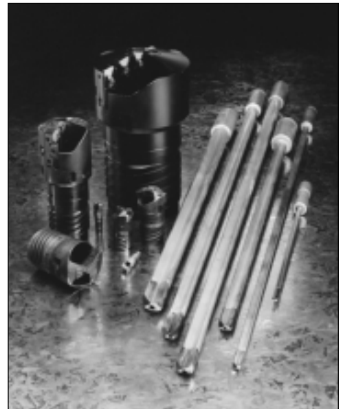
FIGURE 9.15: Deep-hole drilling tools; the gun drills were manufactured by Hyper Tool and the indexable tools were manufactured by Sandvik. (Courtesy TechniDrill Systems, Inc.)
