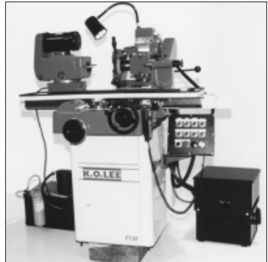
FIGURE 8.12: Tool and cutter grinders, are used to properly sharpen drills and other cutting tools. (Courtesy K. O. Lee Co.)
