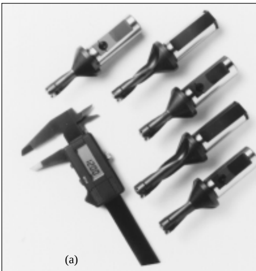
FIGURE 8.17: (a) Indexable drills using Trigon inserts. (b) A Trigon insert and holder. (Courtesy Komet of America, Inc.)
