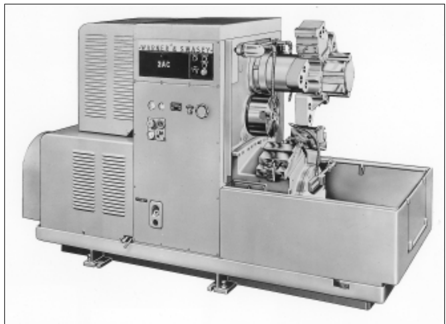
FIGURE 5.9: Single-spindle automatic lathe (Courtesy: National Acme Co., Div. DeVlieg-Bullard Inc.)
