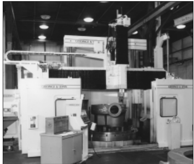
FIGURE 5.8: A vertical turning center machining a heavy part. (Courtesy Giddings & Lewis, LLC)
