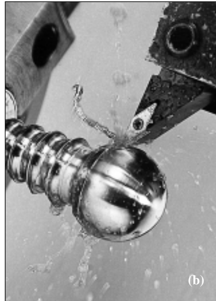
FIGURE 4.3: Chamfering (a) and profiling (b) operations, typically performed on a lathe or a machining center. (Courtesy Valenite Inc.)
