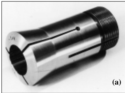
FIGURE 4.14: A collet (a) and a collet mounting assembly (b) are shown here. (Courtesy Lyndex Corp.)
