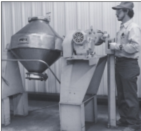
Figure 1.2. Carbide blending equipment, better known as ball mill is used to ensure optimum dispersion of the carbon within the tungsten. (Courtesy American National Carbide Co)
