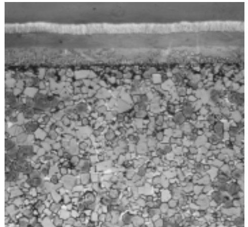
Figure 1.14. Microstructure of a multilayered coated carbide insert at 1500x magnification. (Courtesy of Kennametal Inc.)
