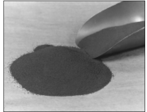
Figure 1.3. Blended tungsten carbide powder is produced by mixing tungsten carbide (WC) with a cobalt (Co) binder in a ball milling process. (Courtesy American National Carbide Co)
