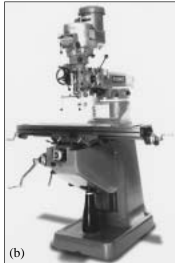
FIGURE 13.3: (a) Stand vertical-spindle column and knee type milling machine. (Courtesy Bridgeport Machinery, Inc.) (b) Three-axis CNC vertical-spindle column and knee type milling machine. (Courtesy Chevalier Machinery, Inc.)
