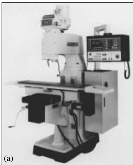
FIGURE 13.3: (a) Stand vertical-spindle column and knee type milling machine. (Courtesy Bridgeport Machinery, Inc.) (b) Three-axis CNC vertical-spindle column and knee type milling machine. (Courtesy Chevalier Machinery, Inc.)
