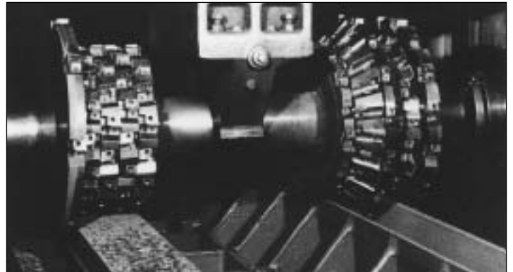
FIGURE 13.29: In gang milling operations, horizontal, vertical, or angular surfaces are machined in one pass. (Courtesy Sandvik Coromant Co.)
