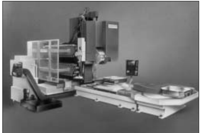
FIGURE 13.14: Machining center with adjustable head, tool magazine and pallet system (Courtesy Cincinnati Machine)
